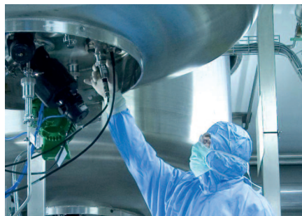
Fig. 1: Left: Glowing steel sample in thermomechanical deformation system for microstructure analysis with LUS. Right: Spectroscopic methods can replace manual handling of samples, which is of particular interest when working with toxic samples or sensitive processes. RECENDT has demonstrated such applications in the PAC-project. Photo credits: Sandoz GmbH.
