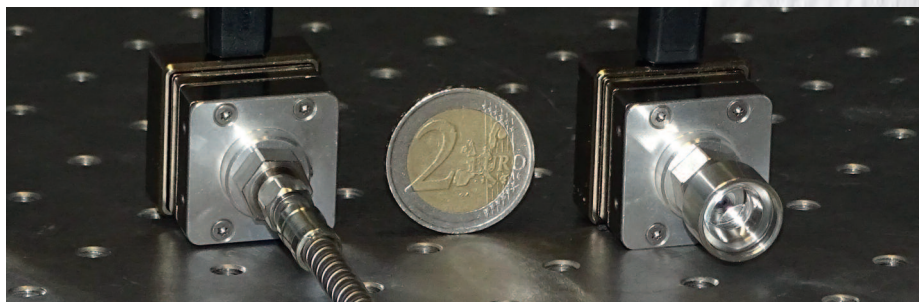
Fig. 1 Photograph of two exemplary microspectrometers, one featuring fibre coupling (left) and one featuring free-space coupling using collimation optics (right). € 2 coin added for scale.
